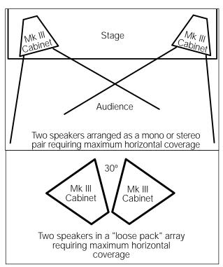
NOTE: When setting up your Mk III Series enclosures, be sure to place the cabinets in such a way as to minimize overlapping radiating patterns.
